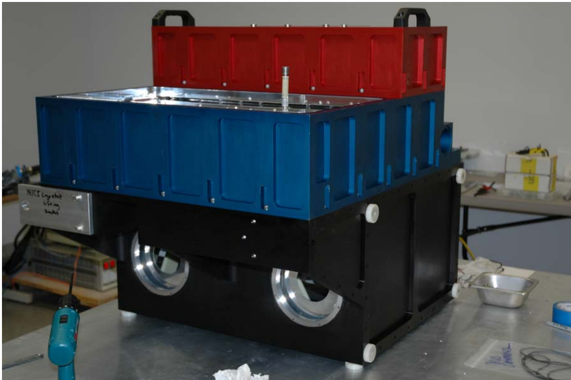
Install the Red Access vacuum jacket cover.
