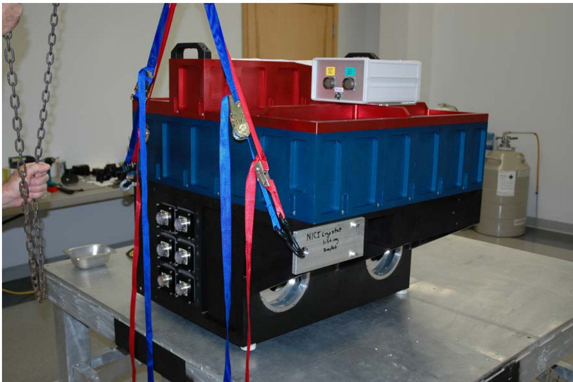
Install the Access Cover Red Detector Vacuum jacket cover.
