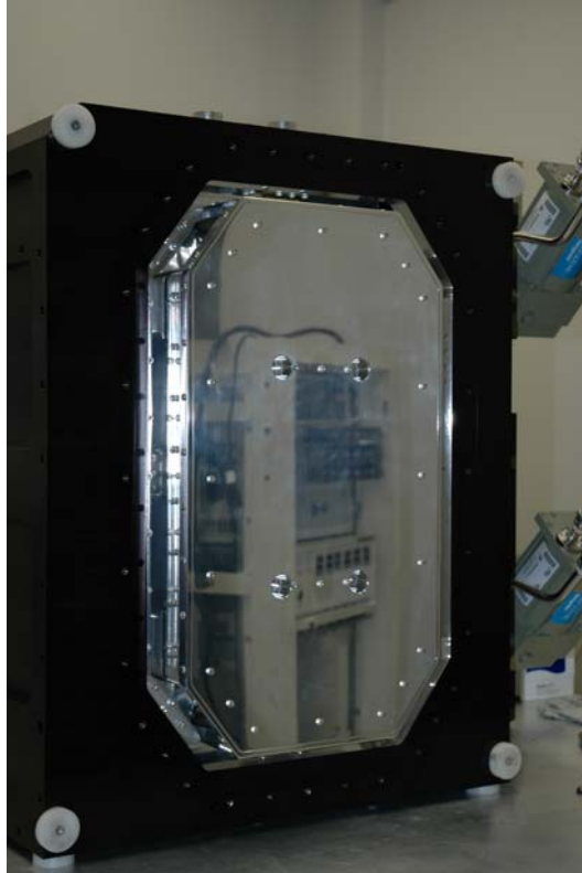
Install Blue Access radiation shield cover.
