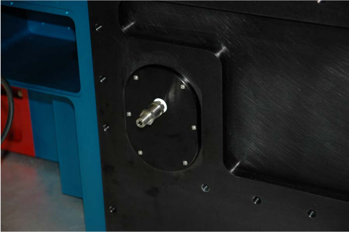
This shows the precharge can cover with check valve.
