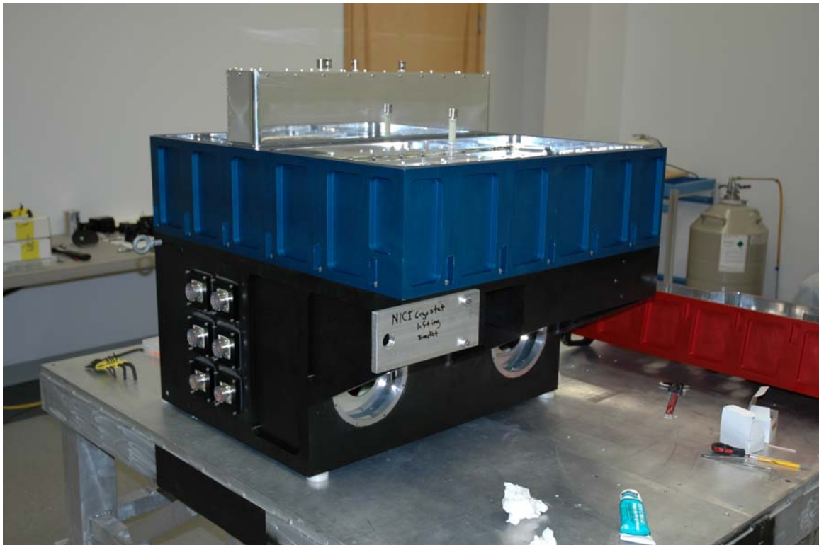
Install the blue vacuum jacket spacer #9408.
