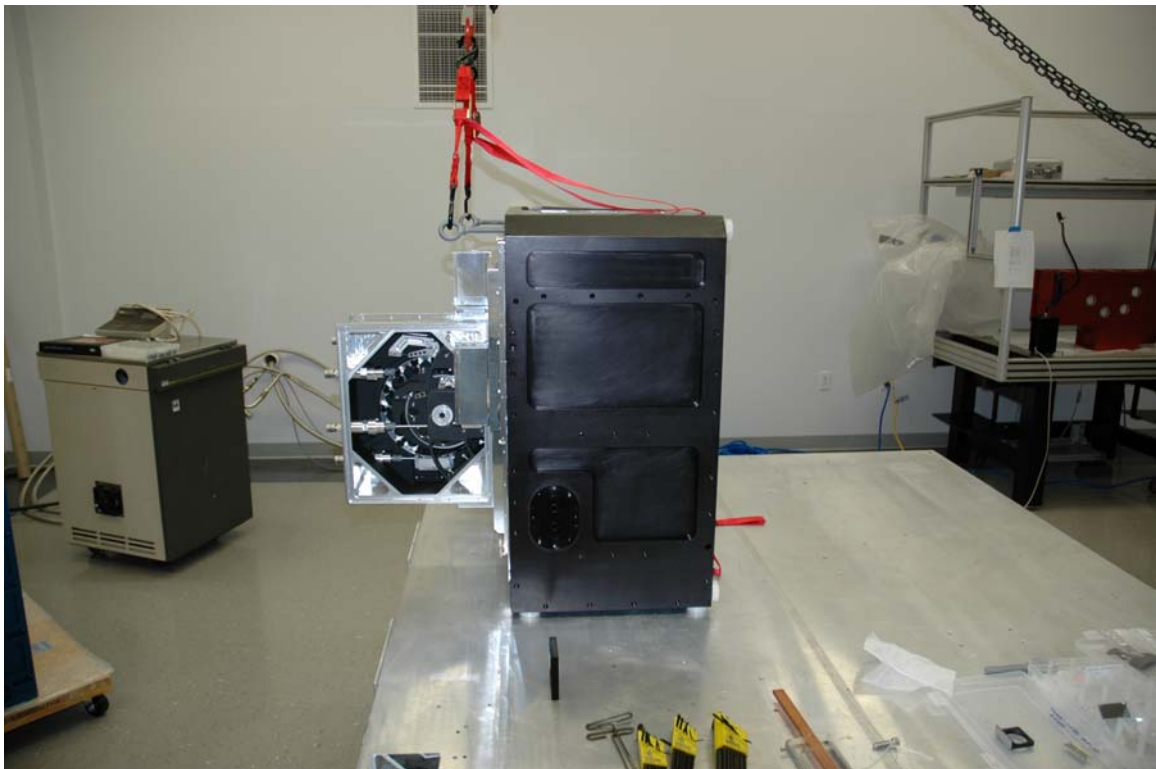
With the mechanism box assembled and mounted the cryostat is tipped to the vertical for the next stages of assembly using the screw eyes in the holes in the vacuum jacket.
