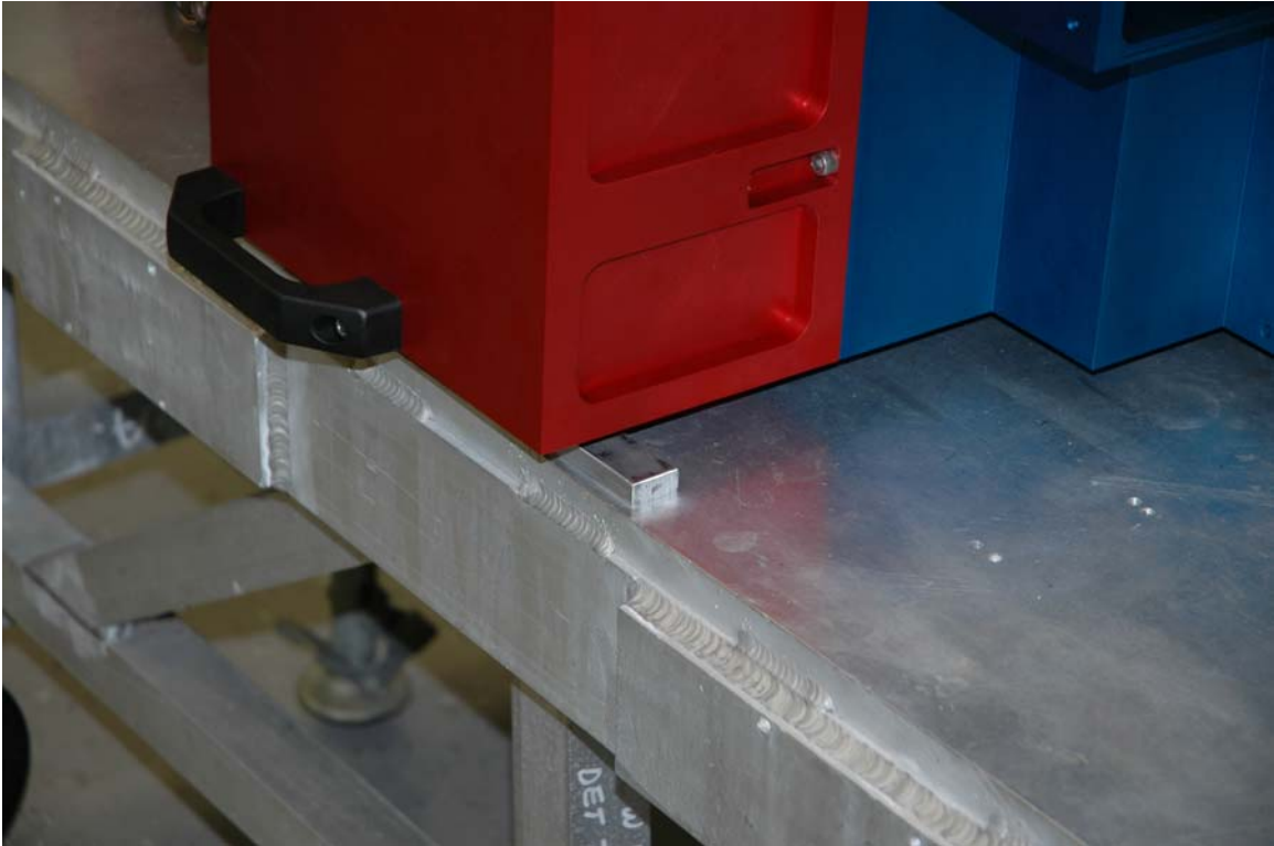
A small spacer is inserted under the red cover to prevent the cryostat from rocking.
