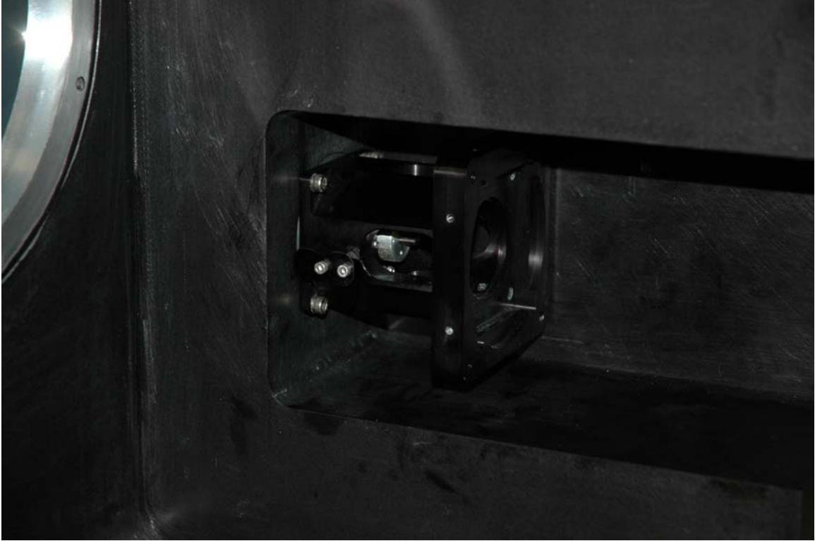
There is one motor mount behind the closed cycle coolers for the Blue filter wheel.
